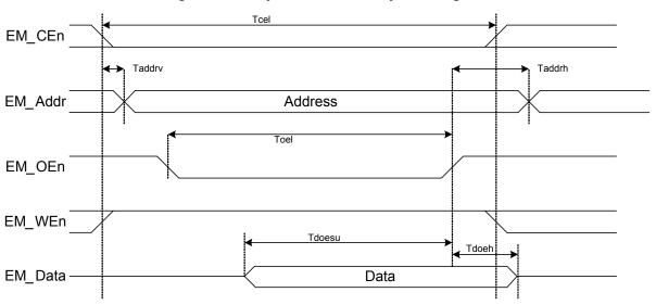
Table 11-63. Asynchronous Read Cycle Specifications
