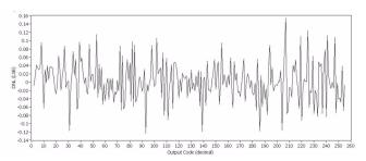
Figure 11-29. IDAC INL vs Temperature, Range = 255  $\mu$ A, Fast Mode
