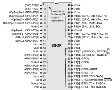
Figure 2-1. 48-pin SSOP Part Pinout
