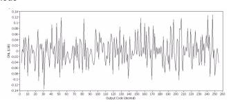
Figure 11-30. IDAC DNL vs Temperature, Range = 255  $\mu$ A, Fast Mode
