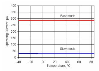
Figure 11-34. IDAC Operating Current vs Temperature, Range = 255 µA, Code = 0, Sink Mode
