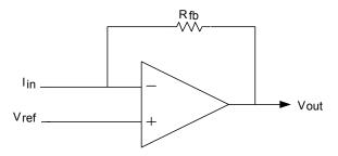
The TIA configuration is used for applications where an external sensor's output is current as a function of some type of stimulus such as temperature, light, magnetic flux etc. In a common application, the voltage DAC output can be connected to the  $V_{\mbox{\scriptsize REF}}$  TIA input to allow calibration of the external sensor bias current by adjusting the voltage DAC output voltage.
