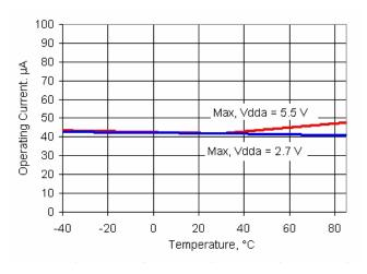
Figure 11-42. VDAC Operating Current vs Temperature, 1 V Mode, Fast Mode
