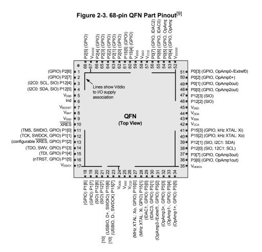
10. Pins are Do Not Use (DNU) on devices without USB. The pin must be left floating.
