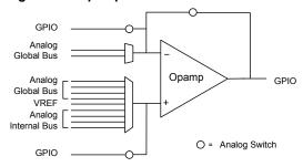
The opamp is uncommitted and can be configured as a gain stage or voltage follower, or output buffer on external or internal signals.
