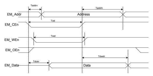
Table 11-64. Asynchronous Write Cycle Specifications
