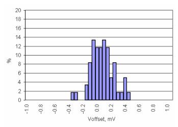
Figure 11-3. Opamp Voffset vs Temperature, Vdda = 5V
