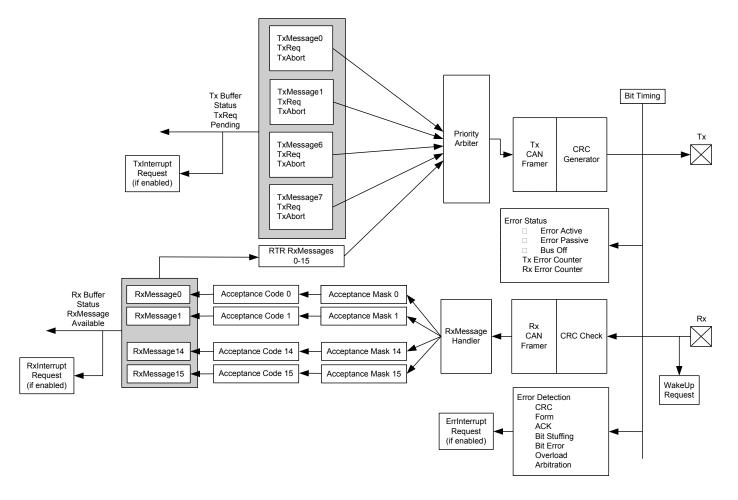
Figure 7-19. CAN Controller Block Diagram
