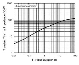
Fig. 6 - Typical Transient Thermal Impedance
