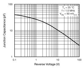
Fig. 5 - Typical Junction Capacitance
