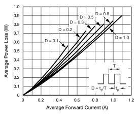
Fig. 2 - Forward Power Loss Characteristics
