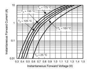
Fig. 3 - Typical Instantaneous Forward Characteristics
