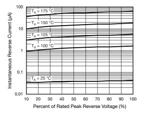
Fig. 4 - Typical Reverse Characteristics
