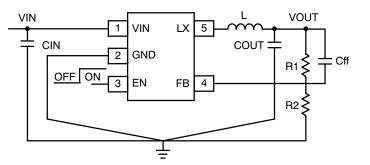
Figure 25. NCP1521 Board Schematic
