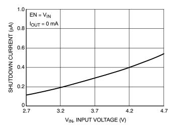
Figure 7. Shutdown Current vs. Supply Voltage
