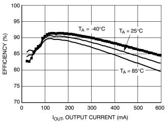
Figure 8. Efficiency vs. Output Current  $(V_{OUT} = 1.8 \text{ V}, V_{IN} = 3.6 \text{ V})$
