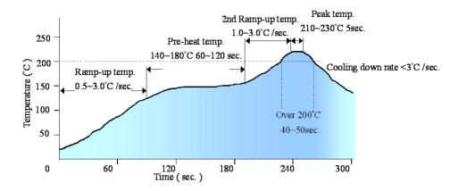
Note: The temperature refers to the pin of filter 7A, measured on the pin 1 (+Vout ) joint.
