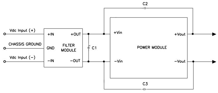
Note: C2 & C3 can be  $0.01\mu$  F to  $0.1\mu$  F. Select the voltage rating to meet input-to-output isolation requirements. C1 should be the recommended value suggested in the power module data sheet.
