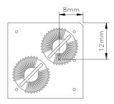
**Figure 5:** Temperature measurement location The allowed maximum hot spot temperature is defined at 115  $^{\circ}$ C
