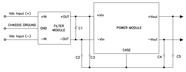
Note: C2 through C5 can be 0.01µ F to 0.1µ F. Select the voltage rating to meet input-to-output isolation requirements. C1 should be the recommended value suggested in the power module data sheet.
