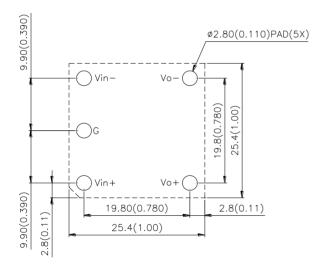
Note: Inside this filter module, the components have no voltage polarity. Hence, the input positive (Vin+) and input negative (Vin-) labels could be swaped for the convenience of layout and matching with power module input connected to the filter module, just remember to swap the output labels accordingly as well. Please refer to Figures 8 and 10 for how it is applied.
