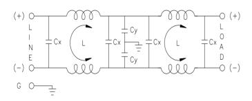
Figure 3: Internal schematics
