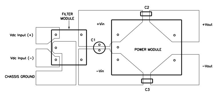
Note: Avoid routing signals or planes under the power module or the filter module. Please ensure all connections are low impedance.
