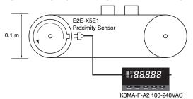
Here, the conveyor belt feed speed is to be displayed in units of  $0.1 \, \text{m/min}$ .
