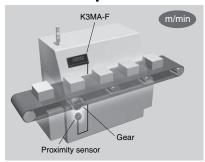
Monitoring line speed for a reflow furnace
