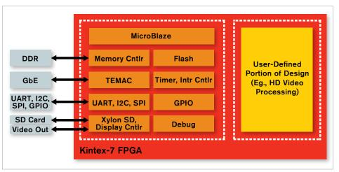
The MicroBlaze™ processor subsystem offers software programmability for high-performance FPGA designs.
