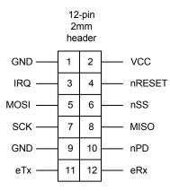
Figure 3-2. CYWM6935PAEC Header Pin-out
