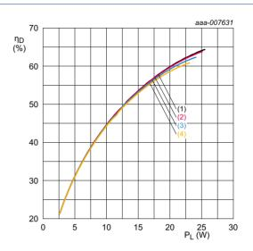
$V_{DS}$  = 28 V;  $I_{Dq}$  = 224 mA; carrier spacing = 5 MHz;  $f_c$  = 960 MHz
