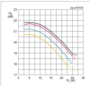
$V_{DS}$  = 28 V;  $I_{Dq}$  = 224 mA; carrier spacing = 5 MHz;  $f_c$  = 960 MHz
