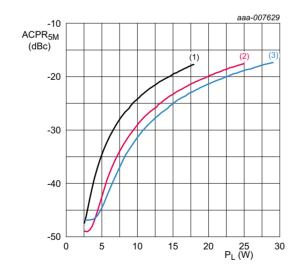
$V_{DS}$  = 28 V;  $I_{Dq}$  = 224 mA; carrier spacing = 5 MHz;  $f_c$  = 960 MHz
