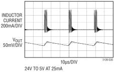
24V TO 5V AT 25mA  $L = 2.2\mu H$   $f_{SW} = 2MHz$  $C_{OUT} = 47\mu F$
