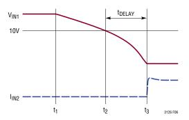
Figure 6. Waveforms During Transition from  $V_{IN1}$  to  $V_{IN2}$
