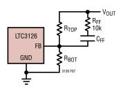
Figure 7. Feedforward Resistor ( $R_{FF}$ ) for Improved Noise Robustness
