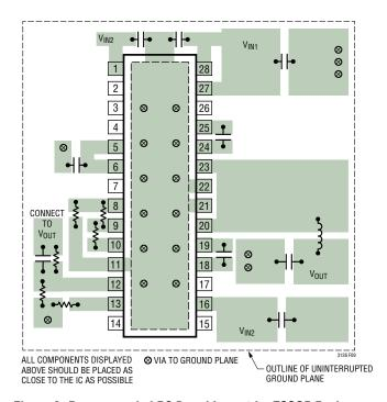
Figure 9. Recommended PC Board Layout for TSSOP Package
