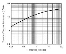
Fig. 6 - Typical Transient Thermal Impedance
