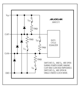
Figure 4. Simplified Clock Input Circuit
