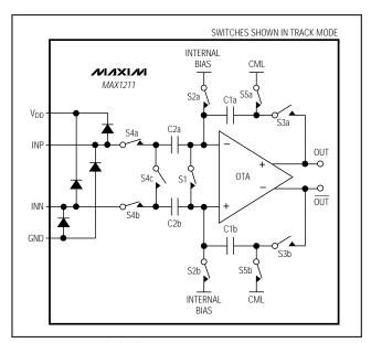
Figure 3. Internal T/H Circuit
