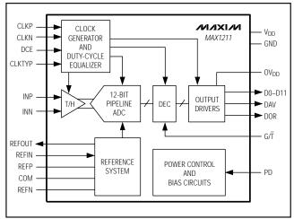
Figure 2. Functional Diagram
