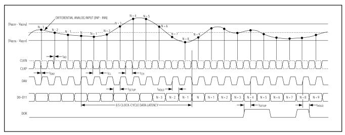
Figure 5. System Timing Diagram
