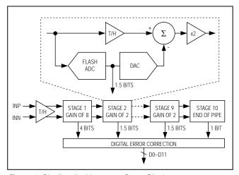
Figure 1. Pipeline Architecture—Stage Blocks
