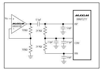
Figure 11. Single-Ended, AC-Coupled Input Drive
