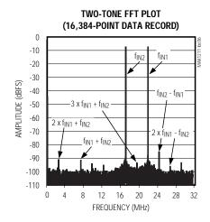
$\begin{array}{l} f_{CLK} = 65.00352 Msps \\ f_{IN1} = 172.5029325 MHz \\ f_{IN2} = 177.50196 MHz \\ SNR = 61.24 dBc \\ SFDR_{TT} = 78.13 dBc \\ IM3 = -81.20 dBc \end{array}$
