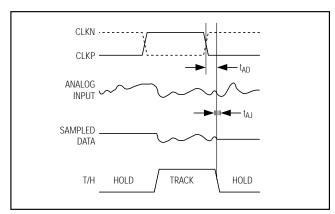
Figure 14. T/H Aperture Timing
