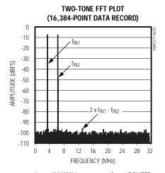
$\begin{array}{l} f_{CLK} = 65.00352 Msps \\ f_{IN1} = 68.4988875 MHz \\ f_{IN2} = 71.49832 MHz \\ SNR = 63.37 dBc \\ SFDR_{TT} = 87.36 dBc \\ IM3 = -88.91 dBc \end{array}$
