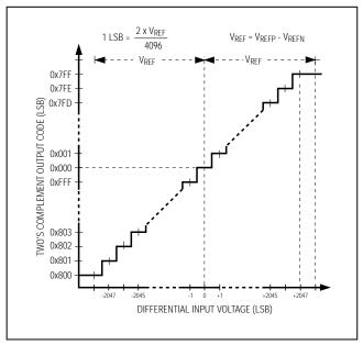
Figure 6. Two's Complement Transfer Function ( $G/\overline{T} = 0$ )
