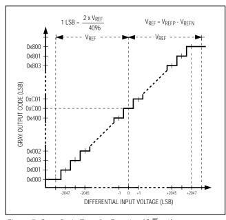
Figure 7. Gray Code Transfer Function ( $G/\overline{T} = 1$ )
