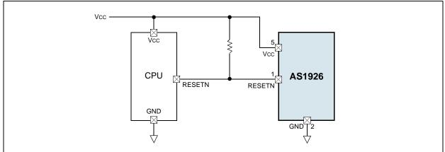
Figure 11. Interfacing to Microprocessors with Bidirectional Reset Pins
