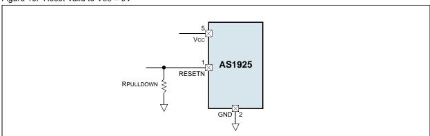
Figure 10. Reset Valid to Vcc = 0V
