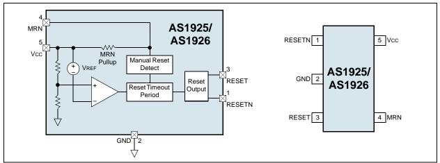
Figure 1. Block Diagram and Pinout
