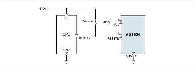
Figure 12. AS1926 Open-Drain RESETN Output with Multiple Supplies
