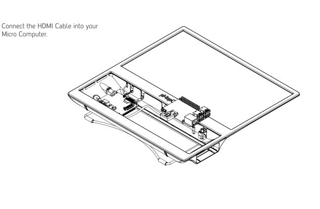
Step 6: Inserting Micro Computer
