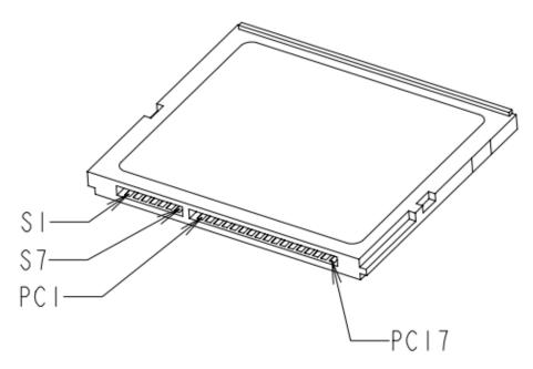
Figure 3-1 Pin Assignment
