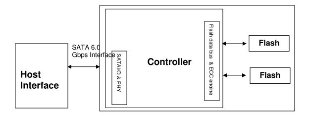
Figure 2-1 Apacer CFast HS block diagram
