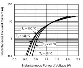
Fig. 3 - Typical Instantaneous Forward Characteristics
