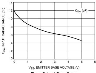
Figure 7. Input Capacitance
