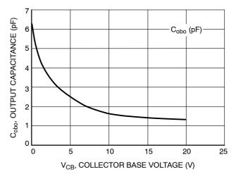
Figure 8. Output Capacitance
