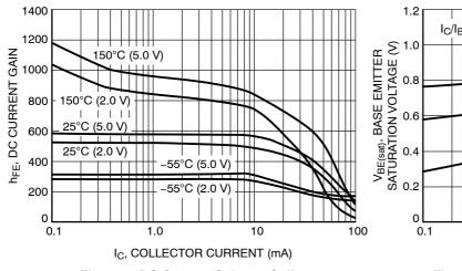
Figure 3. DC Current Gain vs. Collector Current
