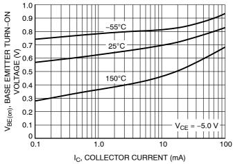
Figure 5. Base Emitter Turn-On Voltage vs.
