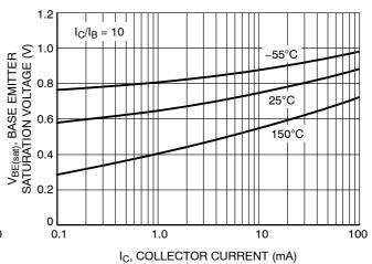
Figure 4. Base Emitter Saturation Voltage vs.
