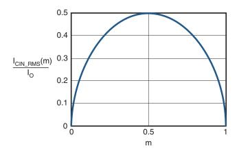
Figure 2. I<sub>CIN</sub> vs. Voltage Conversion Ratio
