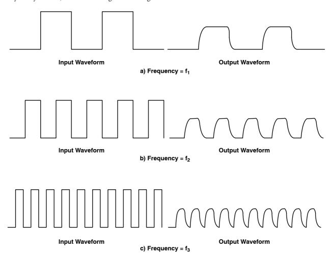
Figure 6. Input and Output Waveforms of Filter
