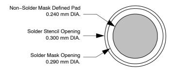
Figure 4. Recommended Non-Solder Mask Defined Pad Illustration
