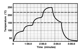
Figure 5. Lead-free (SnAgCu) Solder Ball Reflow Profile
