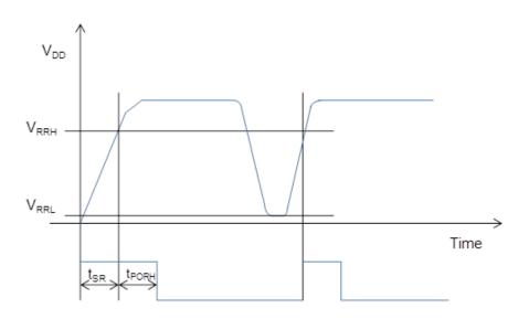
Figure 14. POR Timing Diagram
