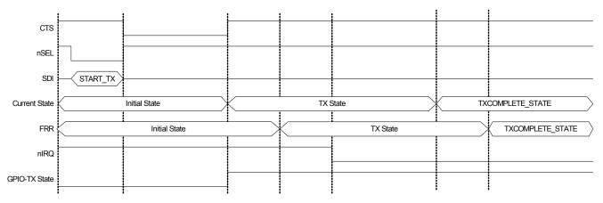
Figure 15. START\_TX Commands and Timing
