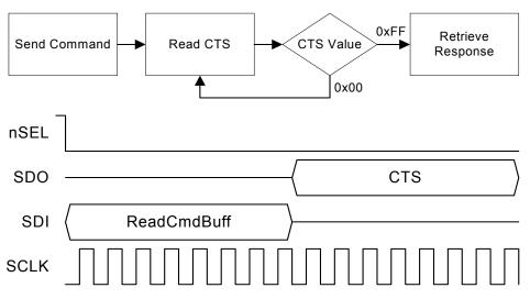
Figure 9. SPI Read Command—Check CTS Value
