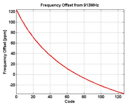
Figure 4. Capacitor Bank Frequency Offset Characteristics
