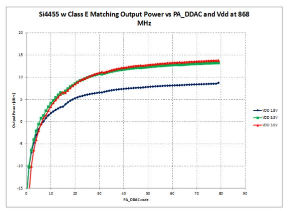
Figure 3. Tx Power vs PA\_PWR\_LVL and VDD
