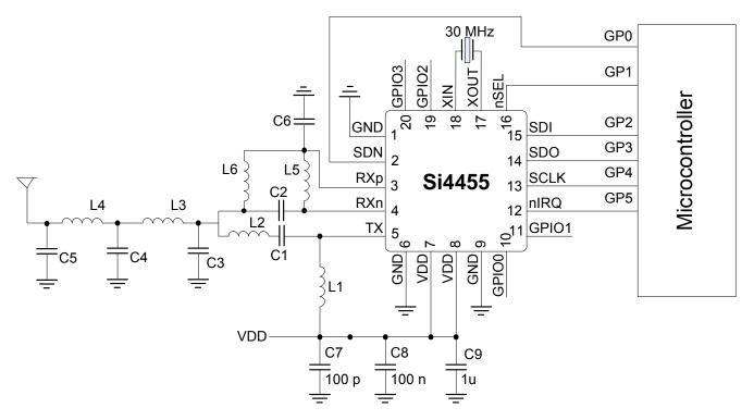
Figure 1. Si4455 Application Circuit
