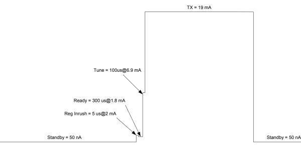
Figure 13. Start-Up Timing and Current Consumption using Standby State
