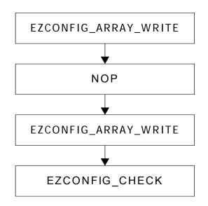
Figure 7. Configuration Command Flowchart
