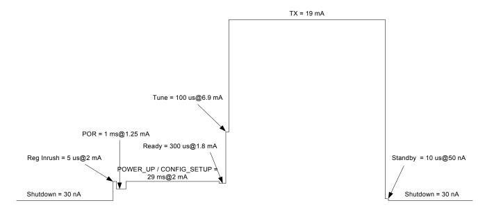
Figure 12. Start-Up Timing and Current Consumption using Shutdown State
