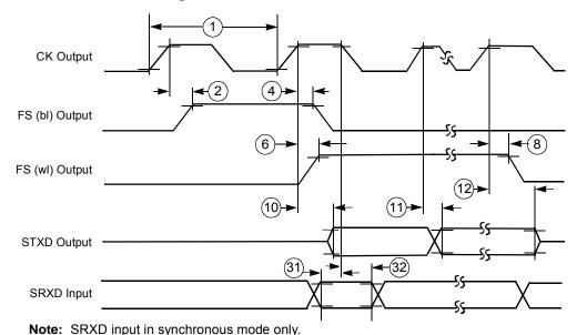
Figure 42. SSI Transmitter Internal Clock Timing Diagram
