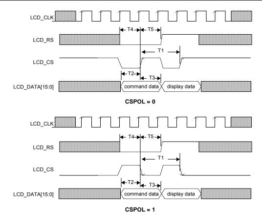
Figure 24. SLCDC Parallel Transfers Timing
