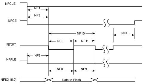
Figure 35. Write Data Latch Timing Dlagram
