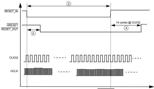
Figure 3. Timing Relationship with RESET\_IN
