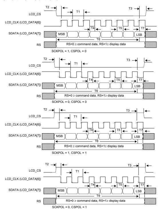
Figure 23. SLCDC Serial Transfer Timing
