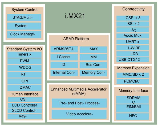
Figure 1. i.MX21 Functional Block Diagram
