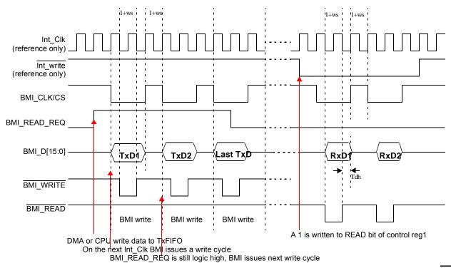
Figure 11. Memory Interface Master Mode, BMI Read/Write to External Slave Device Timing without Wait Signal (MMD\_MODE\_SEL=0, MASTER\_MODE\_SEL=1)
