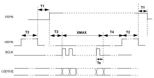
Figure 22. Non-TFT Mode Panel Timing
