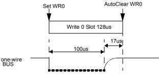
Figure 47. Write 0 Timing
