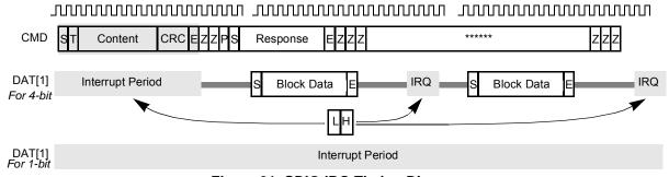
Figure 31. SDIO IRQ Timing Diagram
