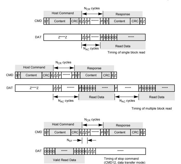
Figure 28. Timing Diagrams at Data Read
