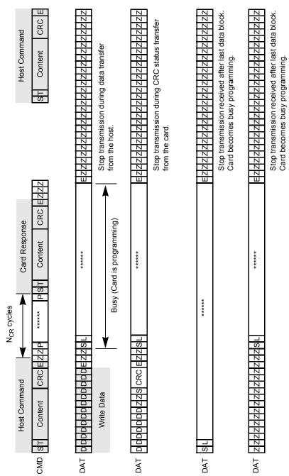
Figure 30. Stop Transmission During Different Scenarios
