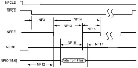
Figure 36. Read Data Latch Timing Diagram
