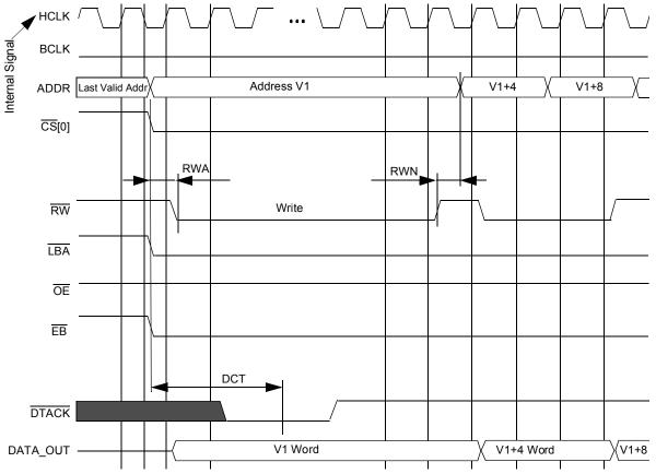
Figure 79. DTACK Level Sensitive Sequential Write <u>Accesses</u>, WSC=2, EW=1, RWA=1, RWN=1, DCT=1, AGE=0 (Example of DTACK Asserting)
