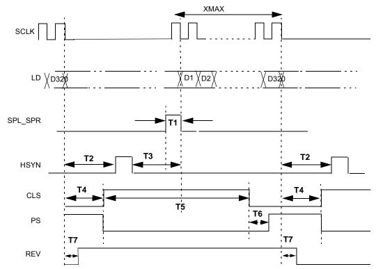
Figure 21. Sharp TFT Panel Timing
