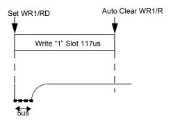
Figure 48. Write 1 Timing
