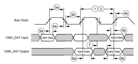
Figure 25. Chip-Select Read Cycle Timing Diagram
