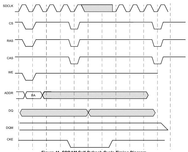
Figure 41. SDRAM Self-Refresh Cycle Timing Diagram
