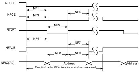
Figure 34. Address Latch Cycle Timing Dlagram
