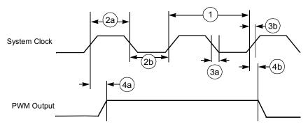
Figure 37. PWM Output Timing Diagram
