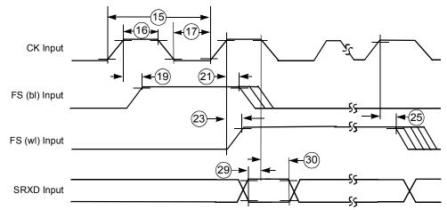
Figure 45. SSI Receiver External Clock Timing Diagram
