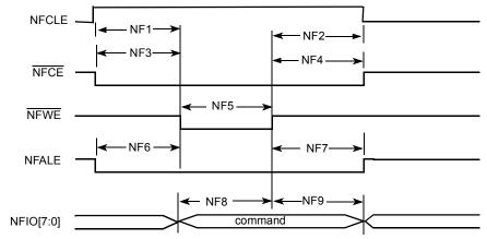
Figure 33. Command Latch Cycle Timing Dlagram
