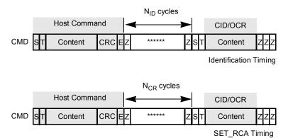
Figure 26. Timing Diagrams at Identification Mode
