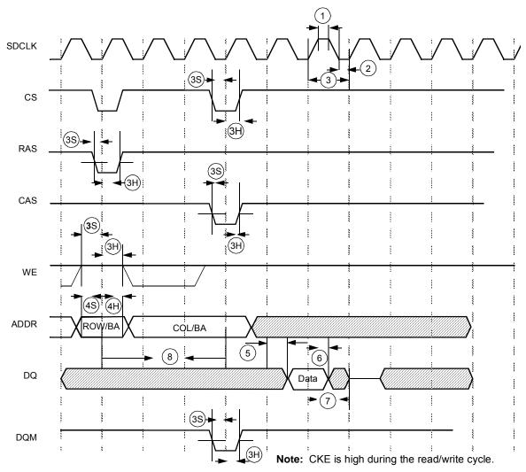
Figure 38. SDRAM Read Cycle Timing Diagram
