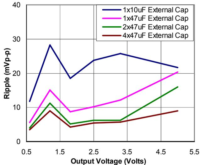
**Note:** Output ripple voltage for various output voltages with external 1x10  $\mu$ F, 1x47  $\mu$ F, 2x47  $\mu$ F or 4x47  $\mu$ F ceramic capacitors at the output (20A load). Input voltage is 12V.
