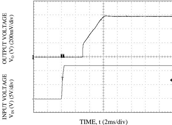
**Start-up Using Input Voltage ( $V_{IN} = 12V$ ,  $I_o = I_{o,max}$ ),
