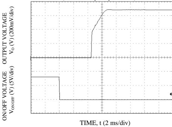
**Start-up Using On/Off Voltage ( $I_o = I_{o,max}$ ),  $V_o=0.69V$**
