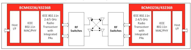
Figure 2: MIMO System Diagram Showing 2 × 2 Antenna Configuration
