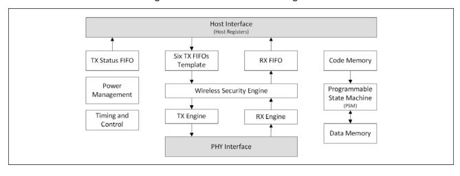
Figure 6: Enhanced MAC Block Diagram
