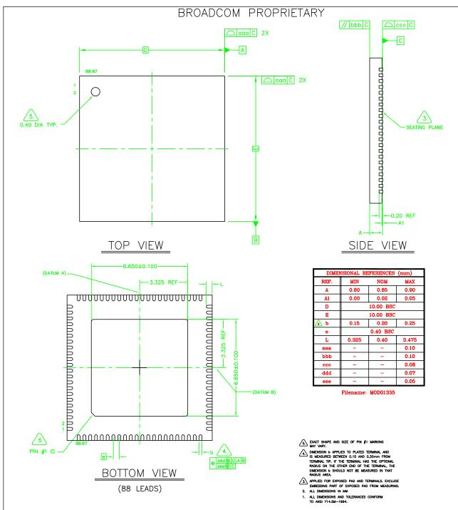
Figure 12: BCM43236/BCM43236B Mechanical Drawing
