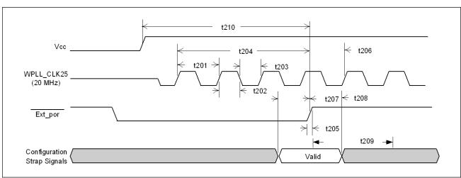
Figure 9: Timing for the Optional External Power-On Reset
