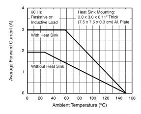
Fig. 1 - Forward Current Derating Curve
