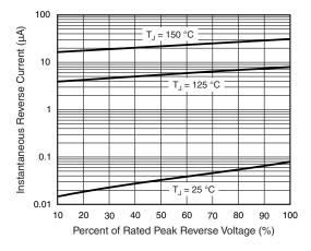
Fig. 4 - Typical Reverse Leakage Characteristics Per Diode
