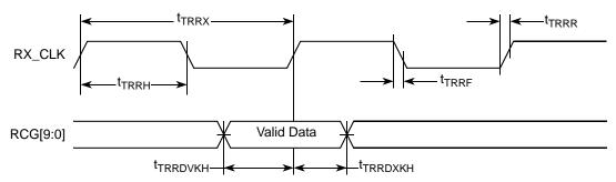
Figure 16. TBI Single-Clock Mode Receive AC Timing Diagram
