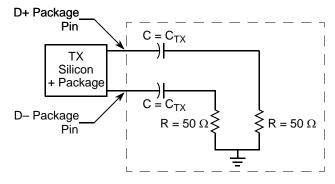
Figure 50. Compliance Test/Measurement Load
