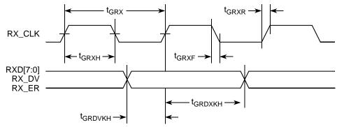
Figure 10. GMII Receive AC Timing Diagram
