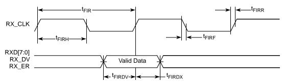
Figure 7. FIFO Receive AC Timing Diagram
