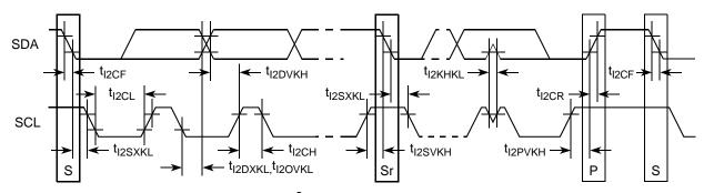
Figure 34. I<sup>2</sup>C Bus AC Timing Diagram
