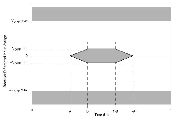
Figure 54. Receiver Input Compliance Mask
