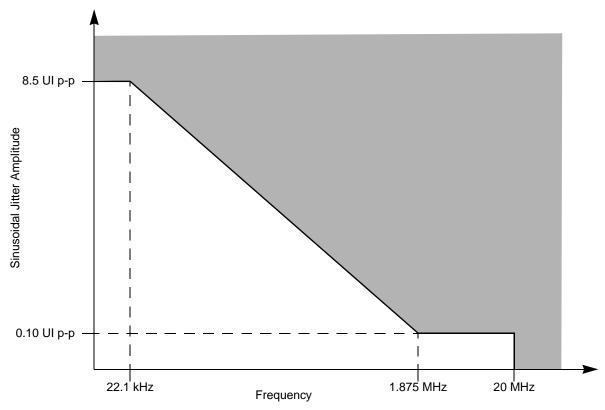
Figure 53. Single Frequency Sinusoidal Jitter Limits
