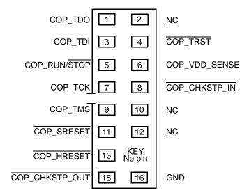
Figure 62. COP Connector Physical Pinout
