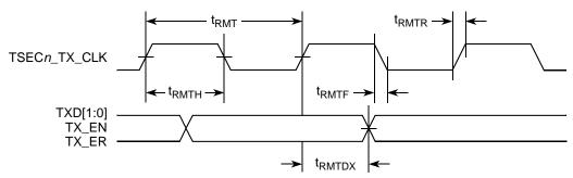
Figure 18. RMII Transmit AC Timing Diagram
