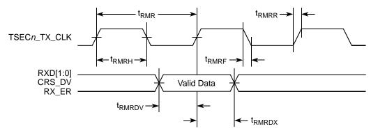
Figure 20. RMII Receive AC Timing Diagram
