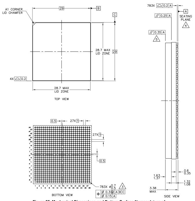
Figure 55. Mechanical Dimensions and Bottom Surface Nomenclature of the HiCTE FC-CBGA and FC-PBGA with Full Lid
