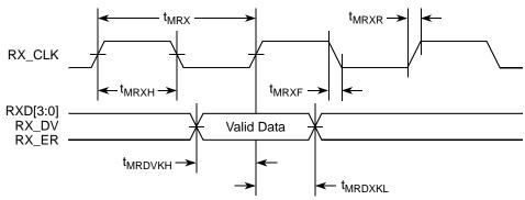
Figure 13. MII Receive AC Timing Diagram
