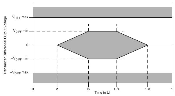
Figure 52. Transmitter Output Compliance Mask
