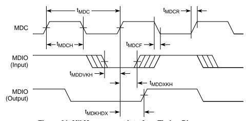
Figure 21. MII Management Interface Timing Diagram
