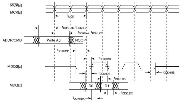
Figure 4. DDR SDRAM Output Timing Diagram
