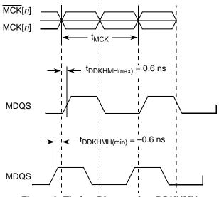
Figure 3. Timing Diagram for tDDKHMH
