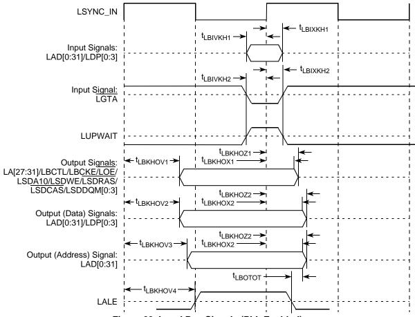
Figure 23. Local Bus Signals (PLL Enabled)
