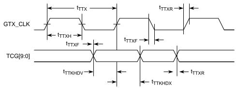
Figure 14. TBI Transmit AC Timing Diagram
