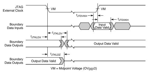
Figure 32. Boundary-Scan Timing Diagram
