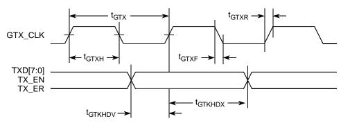
Figure 8. GMII Transmit AC Timing Diagram
