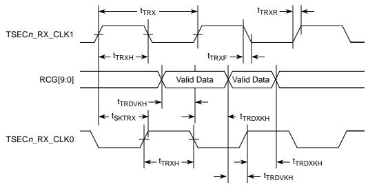
Figure 15. TBI Receive AC Timing Diagram
