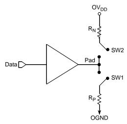
Figure 61. Driver Impedance Measurement
