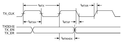
Figure 11. MII Transmit AC Timing Diagram
