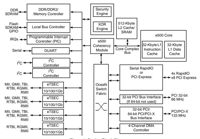
Figure 1. Device Block Diagram
