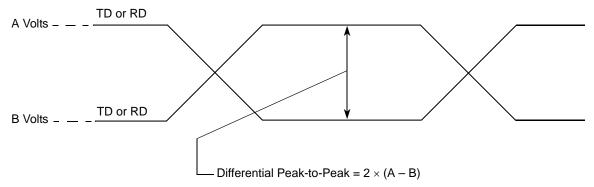
Figure 51. Differential Peak-Peak Voltage of Transmitter or Receiver
