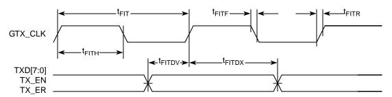
Figure 6. FIFO Transmit AC Timing Diagram
