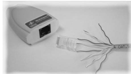
Base unit, RJ45 connector, CAT-5 twisted pair cable
