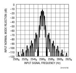
Figure 36. Input Normal Mode Rejection
