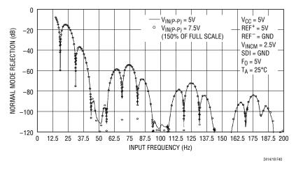
Figure 40. Measured Input Normal Mode Rejection vs Input Frequency with Input Perturbation of 150% Full Scale (50Hz Notch)
