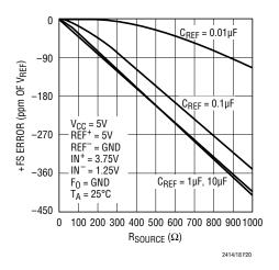
Figure 20. +FS Error vs R<sub>SOURCE</sub> at REF<sup>+</sup> and REF<sup>-</sup> (Large C<sub>REF</sub>)
