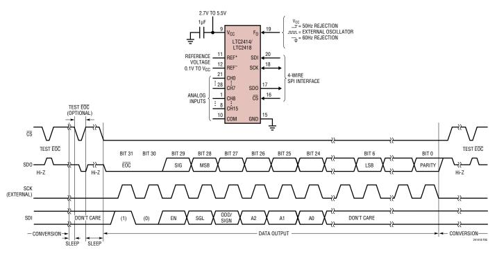
Figure 5. External Serial Clock, Single Cycle Operation
