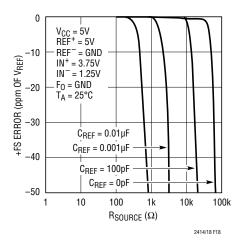
Figure 18. +FS Error vs R<sub>SOURCE</sub> at REF+ or REF- (Small C<sub>IN</sub>)
