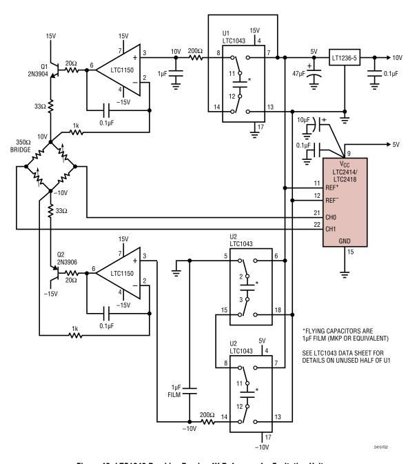
Figure 46. LTC1043 Provides Precise 4X Reference for Excitation Voltages
