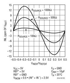
Figure 22. INL vs Differential Input Voltage ( $V_{IN}$  = IN<sup>+</sup> – IN<sup>-</sup>) and Reference Source Resistance ( $R_{SOURCE}$  at REF<sup>+</sup> and REF<sup>-</sup> for Large  $C_{REF}$  Values ( $C_{REF} \ge 1 \mu F$ )
