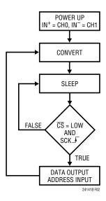
Figure 2. LTC2414/LTC2418 State Transition Diagram
