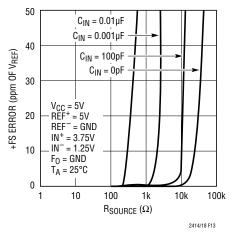
Figure 13. +FS Error vs R<sub>SOURCE</sub> at IN+ or IN- (Small C<sub>IN</sub>)
