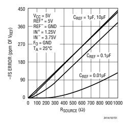
Figure 21. -FS Error vs R<sub>SOURCE</sub> at REF<sup>+</sup> and REF<sup>-</sup> (Large C<sub>REF</sub>)
