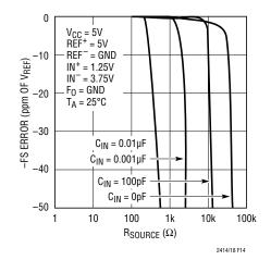
Figure 14. -FS Error vs R<sub>SOURCE</sub> at IN+ or IN- (Small C<sub>IN</sub>)
