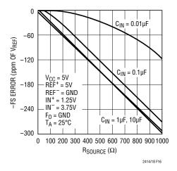
Figure 16. –FS Error vs R<sub>SOURCE</sub> at IN<sup>+</sup> or IN<sup>-</sup> (Large C<sub>IN</sub>)
