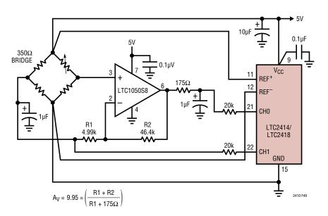
Figure 43. Bridge Amplification Using a Single Amplifier
