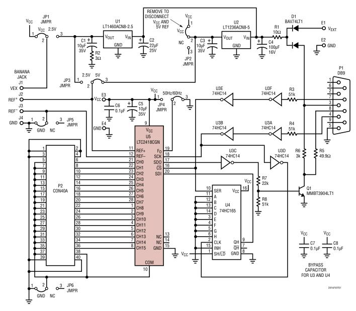
Figure 51. Demo Board Schematic
