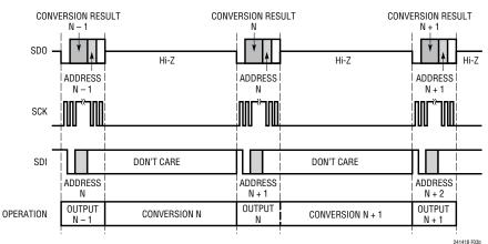
Figure 3b. Typical Operation Sequence
