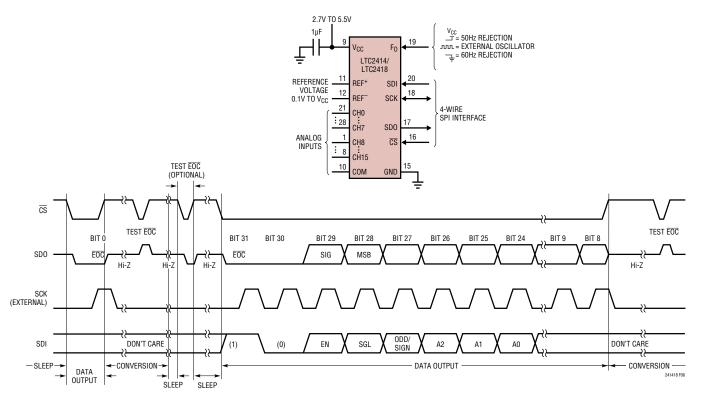
Figure 6. External Serial Clock, Reduced Data Output Length
