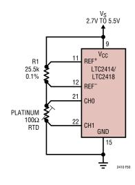
Figure 44. Remote Half Bridge Interface
