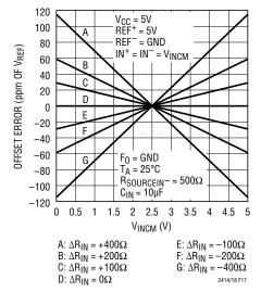
Figure 17. Offset Error vs Common Mode Voltage ( $V_{INCM} = IN^+ = IN^-$ ) and Input Source Resistance Imbalance ( $\Delta R_{IN} = R_{SOURCEIN} + - R_{SOURCEIN}$ ) for Large  $C_{IN}$  Values ( $C_{IN} \ge 1\mu F$ )
