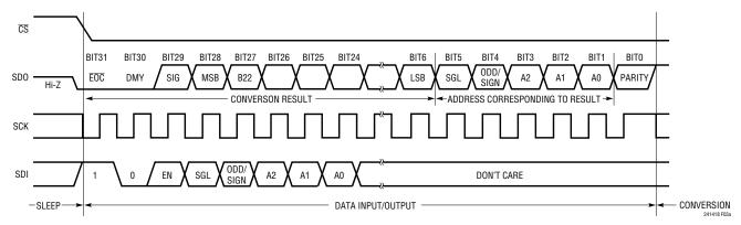
Figure 3a. Input/Output Data Timing
