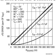
Figure 15. +FS Error vs R<sub>SOURCE</sub> at IN<sup>+</sup> or IN<sup>-</sup> (Large C<sub>IN</sub>)
