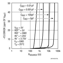
Figure 19. -FS Error vs R<sub>SOURCE</sub> at REF+ or REF- (Small C<sub>IN</sub>)
