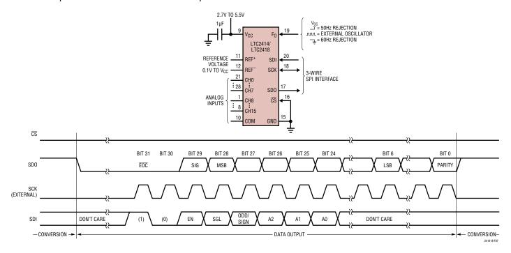
Figure 7. External Serial Clock,  $\overline{CS} = 0$  Operation
