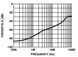
FIGURE 36. CHANNEL-TO-CHANNEL CROSSTALK - DUALS AND QUADS (WORST CHANNEL)
