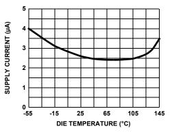
FIGURE 40. SUPPLY CURRENT - OFF (PER AMP) vs DIE TEMPERATURE
