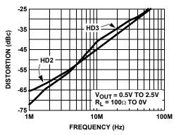
FIGURE 34. 2nd AND 3rd HARMONIC DISTORTION vs FREQUENCY
