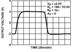
FIGURE 21. LARGE SIGNAL PULSE RESPONSE (SPLIT SUPPLIES)
