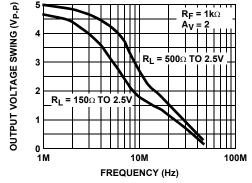
FIGURE 17. OUTPUT VOLTAGE SWING vs FREQUENCY FOR THD < 1\%
