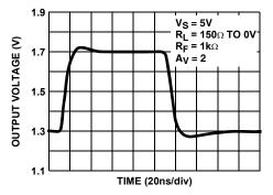
FIGURE 20. SMALL SIGNAL PULSE RESPONSE (SINGLE SUPPLY)
