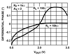
FIGURE 30. DIFFERENTIAL PHASE FOR RL TIED TO 0V
