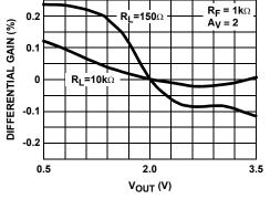
FIGURE 29. DIFFERENTIAL GAIN FOR  $\rm R_L$  TIED TO 0V
