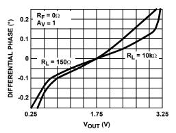
FIGURE 26. DIFFERENTIAL PHASE FOR RL TIED TO 0V
