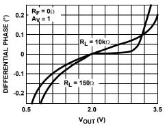
FIGURE 28. DIFFERENTIAL PHASE FOR RL TIED TO 2.5V
