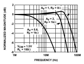
FIGURE 1. NON-INVERTING FREQUENCY RESPONSE (GAIN)
