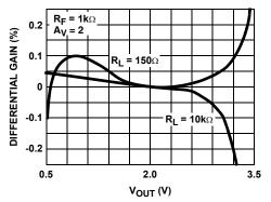
FIGURE 31. DIFFERENTIAL GAIN FOR  $\rm R_L$  TIED TO 2.5V
