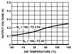
FIGURE 42. NEGATIVE OUTPUT VOLTAGE SWING vs DIE TEMPERATURE
