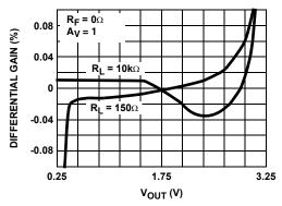
FIGURE 25. DIFFERENTIAL GAIN FOR RL TIED TO 0V
