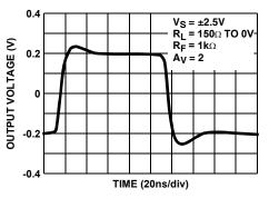
FIGURE 22. SMALL SIGNAL PULSE RESPONSE (SPLIT SUPPLY)
