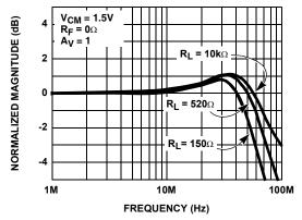
FIGURE 7. FREQUENCY RESPONSE FOR VARIOUS RL
