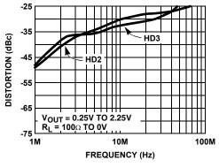
FIGURE 33. 2nd AND 3rd HARMONIC DISTORTION vs FREQUENCY
