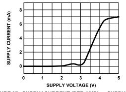
FIGURE 37. SUPPLY CURRENT (PER AMP) vs SUPPLY VOLTAGE
