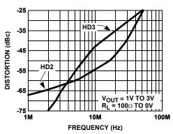
FIGURE 35. 2nd AND 3rd HARMONIC DISTORTION vs FREQUENCY
