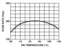
FIGURE 24. SLEW RATE vs DIE TEMPERATURE
