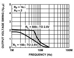
FIGURE 18. OUTPUT VOLTAGE SWING vs FREQUENCY FOR THD < 0.1%
