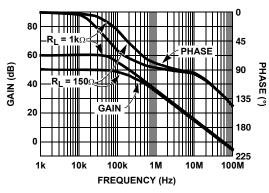
FIGURE 11. OPEN LOOP GAIN AND PHASE vs FREQUENCY
