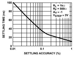
FIGURE 23. SETTLING TIME vs SETTLING ACCURACY
