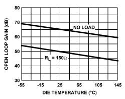
FIGURE 12. OPEN LOOP VOLTAGE GAIN vs DIE TEMPERATURE
