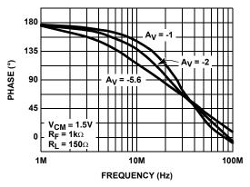
FIGURE 4. INVERTING FREQUENCY RESPONSE (PHASE)
