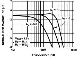
FIGURE 3. INVERTING FREQUENCY RESPONSE (GAIN)
