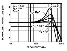
FIGURE 8. FREQUENCY RESPONSE FOR VARIOUS CL
