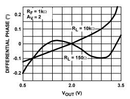
FIGURE 32. DIFFERENTIAL PHASE FOR RL TIED TO 2.5V
