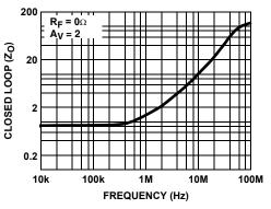
FIGURE 14. CLOSED LOOP OUTPUT IMPEDANCE vs FREQUENCY
