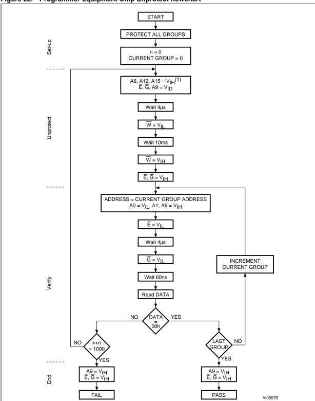
Figure 22. Programmer Equipment Chip Unprotect flowchart
