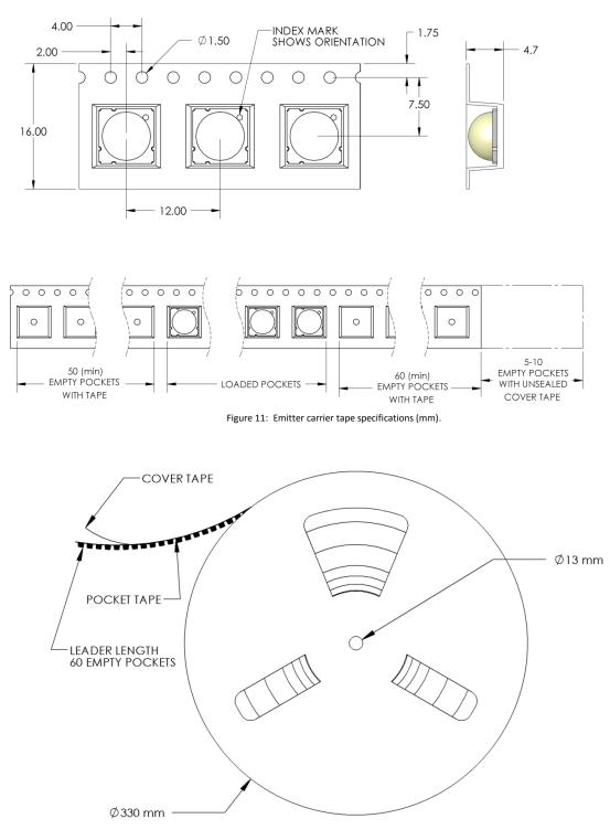
Figure 12: Emitter Reel specifications (mm).
