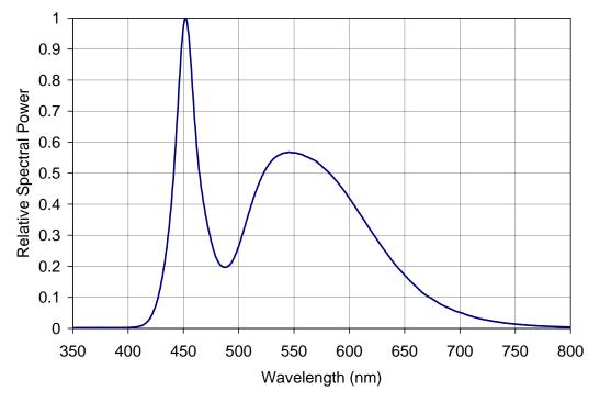
Figure 5: Typical relative spectral power vs. wavelength @  $T_C = 25^{\circ}C$
