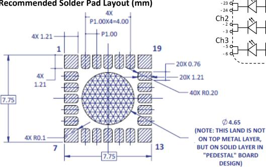
Figure 2a: Recommended solder pad layout for anode, cathode, and thermal pad.
