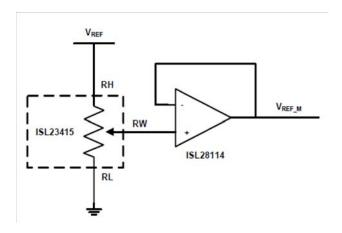
FIGURE 2. V<sub>REF</sub> ADJUSTMENT
