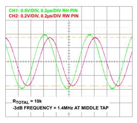
FIGURE 23. 10k -3dB CUT OFF FREQUENCY
