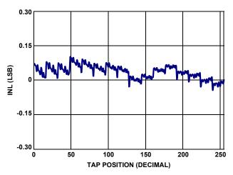
FIGURE 6. 50k INL vs TAP POSITION, V<sub>CC</sub> = 5V
