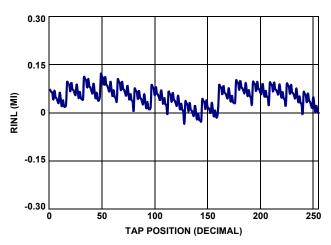
FIGURE 10. 50k RINL vs TAP POSITION, V<sub>CC</sub> = 5V
