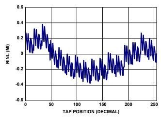
FIGURE 9. 10k RINL vs TAP POSITION, V<sub>CC</sub> = 5V
