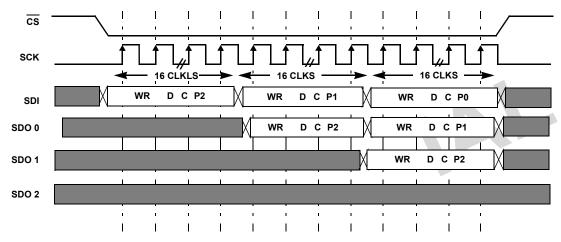
FIGURE 30. DAISY CHAIN WRITE SEQUENCE OF N = 3 DCP
