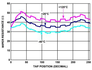
FIGURE 12. 50k WIPER RESISTANCE vs TAP POSITION,  $V_{CC} = 5V$
