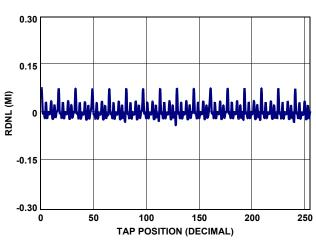
FIGURE 8. 50k RDNL vs TAP POSITION,  $V_{CC} = 5V$
