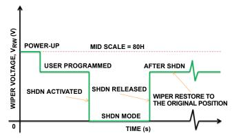
FIGURE 26. SHUTDOWN MODE WIPER RESPONSE
