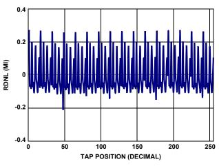
FIGURE 7. 10k RDNL vs TAP POSITION, V<sub>CC</sub> = 5V
