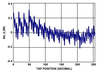
FIGURE 5. 10k INL vs TAP POSITION, V<sub>CC</sub> = 5V
