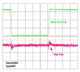
FIGURE 19. WIPER DIGITAL FEEDTHROUGH
