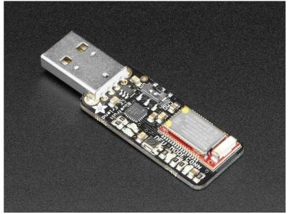
In it's simplest form, it works on the same principle as a common USB/Serial adapter (the <u>FTDI Friend</u> (http://adafru.it/dQa), for example!). Any data that you enter via your favorite terminal emulator on your development machine will be transferred over the air to the connected phone or tablet, and vice versa.
