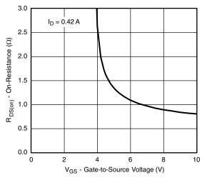
On-Resistance vs. Gate-to-Source Voltage
