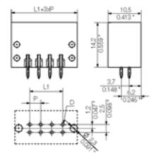
1729470000 S2L 3.5/14/180F3.5SN OR PCB plug-in connector, Male connectors, Soldered connection, Pitch: 3.50 mm, No. of poles: 14, 180°, Box 4032248040896 50 pc(s).
