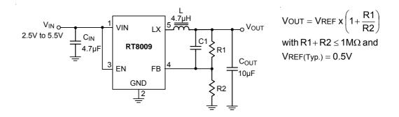
Figure 2. Adjustable Voltage Regulator
