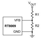
Figure 4. Setting the Output Voltage
