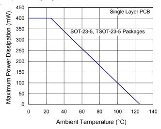
Figure 5. Derating Curves for RT8009 Package
