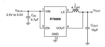
Figure 1. Fixed Voltage Regulator
