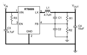
Figure 6. EVB Schematic
