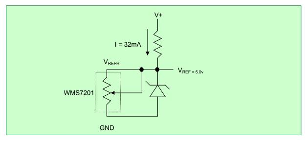
FIGURE 10 - WMS7201 TRIMMING VOLTAGE REFERENCE
