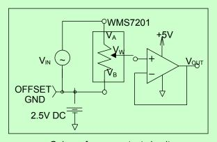
Gain vs. frequency test circuit
