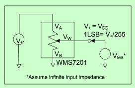
Potentiometer divider nonlinearity error test circuit (INL, DNL)
