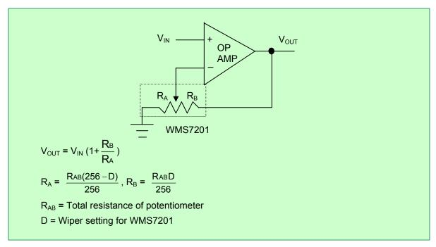
FIGURE 9 - PROGRAMMABLE NON-INVERTING GAIN AMPLIFIER USING THE WMS7201
