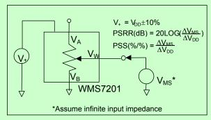
Power supply sensitivity test circuit (PSS, PSRR)
