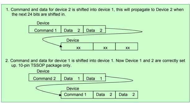
FIGURE 4 - DAISY CHAIN COMMAND EXAMPLE
