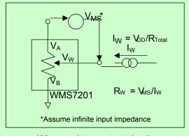
Wiper resistance test circuit
