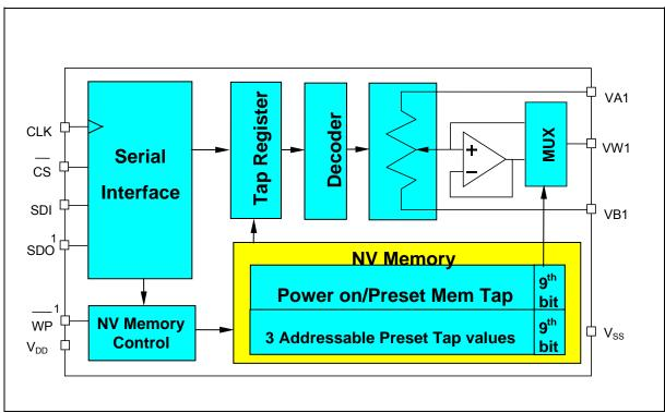
FIGURE 1 - WMS7201 BLOCK DIAGRAM
