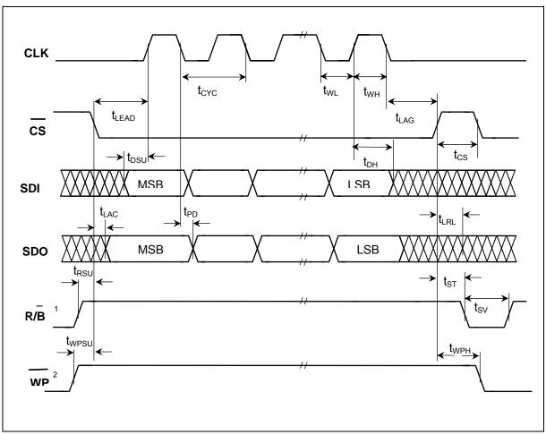
FIGURE 6 - WMS7201 TIMING DIAGRAM
