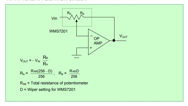
FIGURE 8 - PROGRAMMABLE INVERTING GAIN AMPLIFIER USING THE WMS7201
