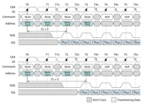
Notes: 1.  $D_{OUT}n$  (or x, b, g) = data-out from column n (or column x, column b, column g).
