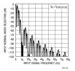
Figure 33. Input Normal Mode Rejection at DC
