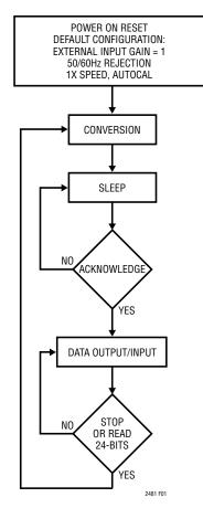
Figure 1. LTC2481 State Transition Diagram
