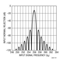
Figure 41. Input Normal Mode Rejection 2x Speed Mode
