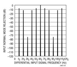
Figure 31. Input Normal Mode Rejection, Internal Oscillator and 50Hz Notch Mode
