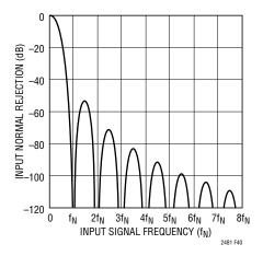
Figure 40. Input Normal Mode Rejection 2x Speed Mode
