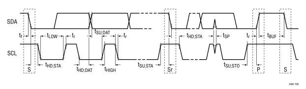
Figure 2. Definition of Timing for F/S-Mode Devices on the I<sup>2</sup>C-Bus
