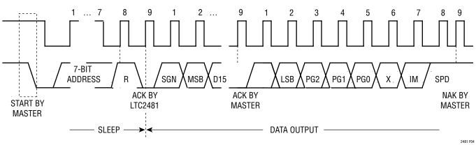
Figure 4. Timing Diagram for Reading from the LTC2481
