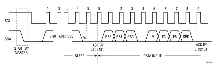
Figure 3. Timing Diagram for Writing to the LTC2481
