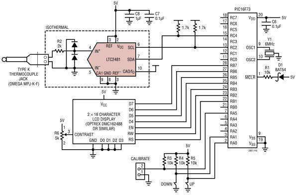
Figure 45. Complete Type K Thermocouple Meter
