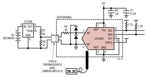
Figure 44. Calibration Setup
