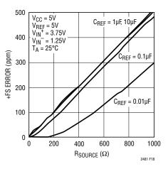
Figure 18. +FS Error vs R<sub>SOURCE</sub> at REF<sup>+</sup> or REF<sup>-</sup> (Large C<sub>REF</sub>)
