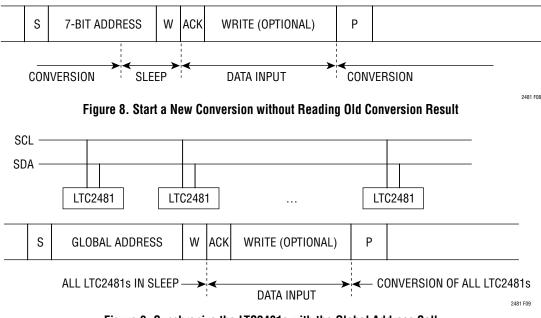
Figure 9. Synchronize the LTC2481s with the Global Address Call
