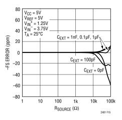
Figure 15. –FS Error vs R<sub>SOURCE</sub> at IN<sup>+</sup> and IN<sup>-</sup>
