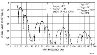
Figure 39. Measured Input Normal Mode Rejection vs Input Frequency with Input Perturbation of 150% Full-Scale (50Hz Notch)
