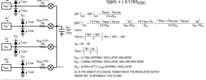
$\begin{array}{l} \mbox{SWITCHING FREQUENCY} \\ \mbox{f}_{SW} = 123 \mbox{kHz INTERNAL OSCILLATOR} \\ \mbox{f}_{SW} = 0.4 \bullet \mbox{f}_{EOSC} \mbox{EXTERNAL OSCILLATOR} \end{array}$
