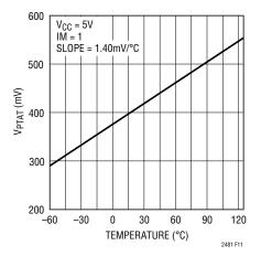
Figure 11. Internal PTAT Signal vs Temperature
