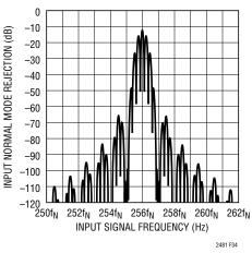
Figure 34. Input Normal Mode Rejection at  $f_s = 256 f_N$
