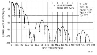
Figure 36. Input Normal Mode Rejection vs Input Frequency with Input Perturbation of 100% Full-Scale (50Hz Notch)
