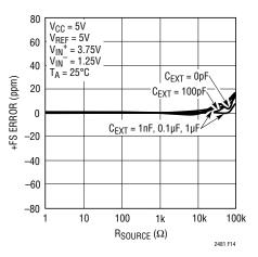
Figure 14. +FS Error vs R<sub>SOURCE</sub> at IN<sup>+</sup> and IN<sup>-</sup>
