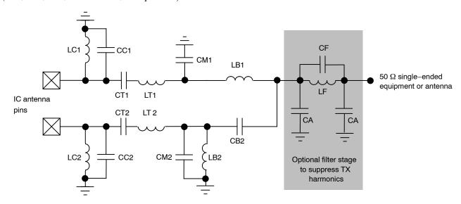
Figure 9. Structure of the Differential Antenna Interface for TX/RX Operation to 50  $\Omega$  Single-ended Equipment or Antenna
