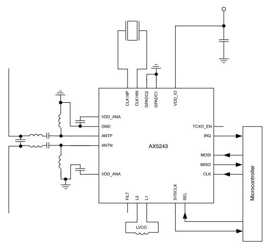
Figure 12. Typical Application Diagram with External VCO Inductor
