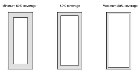
Figure 18. Solder Paste Application on Pins
