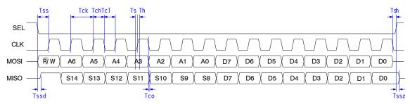
Figure 6. SPI 8 Bit Read/Write Access with Timing
