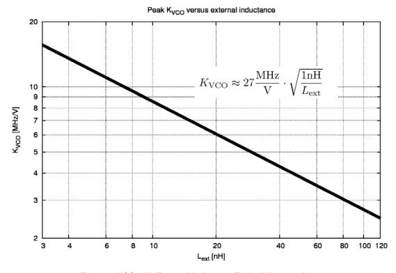
Figure 4. VCO with External Inductors: Typical  $K_{\text{VCO}}$  vs.  $L_{\text{ext}}$
