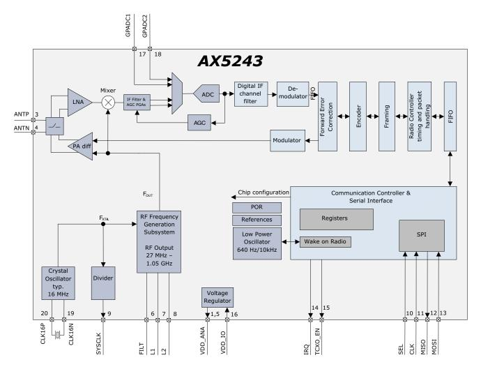
Figure 1. Functional Block Diagram of the AX5243
