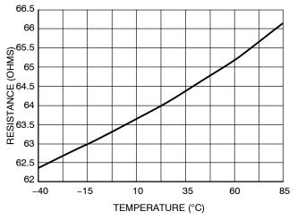
Figure 3. Typical Resistance over Temperature
