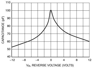
Figure 4. Typical Line Capacitance over Reverse Voltage
