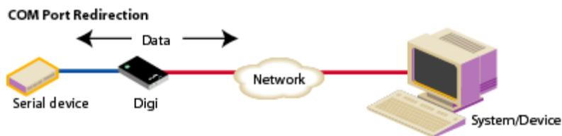
The network is transparent to both the application and the serial device.
