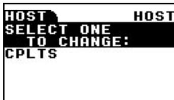
3. Move cursor position using the **Up** (Left) and **Dn** (Right) keys. Once you position the cursor to the item you want to change, press the **Sel** key to enter the editing submenu.
