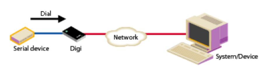
Modem dial-in and bi-directional options provide a login from the Digi device. See [Assign a profile to a serial port](#) for more information.
