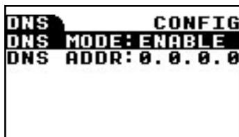
4. Set the IP address of the DNS server in the same manner as setting the IP address.
