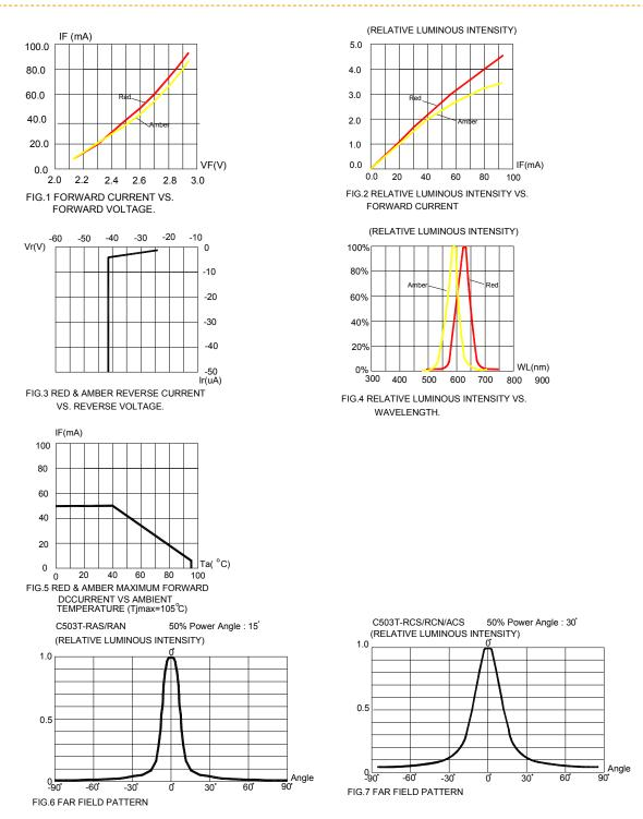
The above data are collected from statistical figures that do not necessarily correspond to the actual parameters of each single LED. Hence, these data will be changed without further notice.
