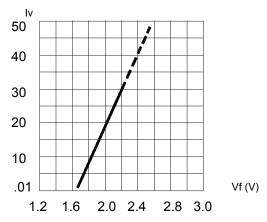
Fig. 3 Relative Intensity (10mA) vs. Forward Voltage
