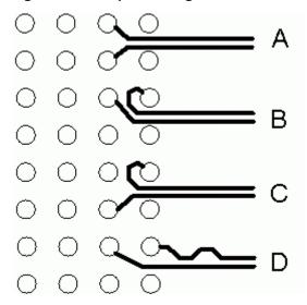
Figure 26: Differential Skew Matching Serpentine
