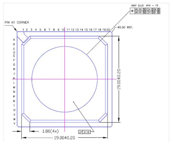
Figure 2: Package - Top View
