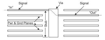
Figure 18: Signal Through a Via
