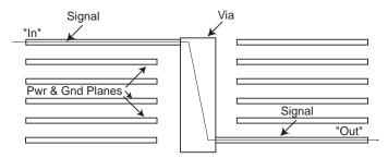
Because of the high frequencies present in the RapidIO signal, vias become a significant contributor to signal degradation. Most vias are formed by a cylinder going through the PCB board. Because the via has some length, there is an inductance associated with the via. Parasitic capacitance comes from the power and ground planes through which the via passes. From this structure, the model of the vias in RLC lumps as shown in Figure 19 and Figure 20.
