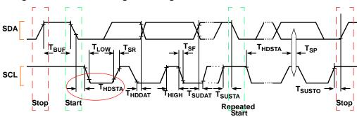
Figure 6: I<sup>2</sup>C Interface Signal Timings
