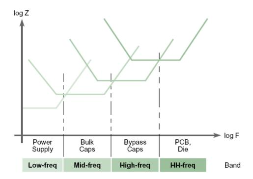
Figure 34: Decoupling Bypass Frequency Bands
