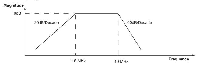
Figure 5: Weighing function for RMS Phase Jitter Calculation
