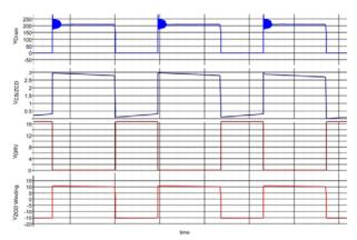
Figure 9. ZCD Winding Waveforms
