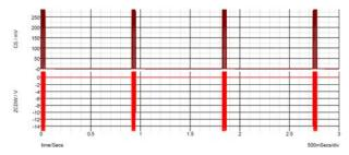
Figure 12. Output Short Detection and Protection
