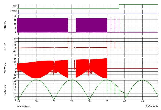
Figure 7. Secondary Side Winding Short-Circuit Waveforms
