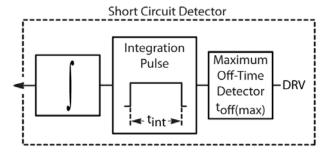
Figure 11. Output Short-Circuit Detector
