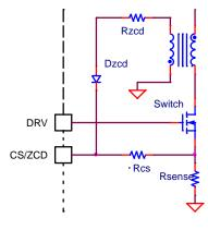
Figure 8. ZCD Winding Implementation
