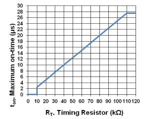
Figure 5. Maximum On-Time vs R<sub>T</sub>
