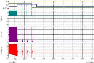
Figure 10. Overvoltage Detection Operating Waveforms
