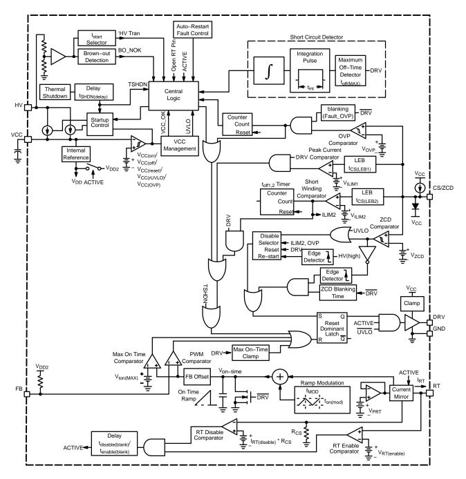
Figure 2. NCL30060 Internal Functional Block Diagram
