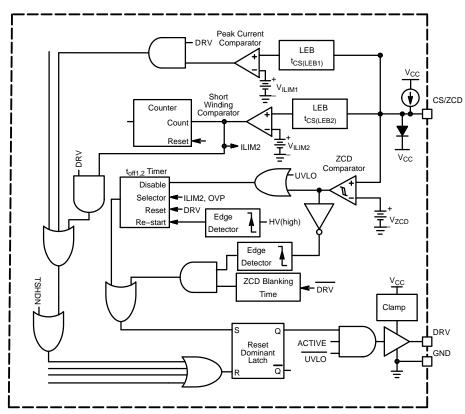
Figure 6. Current Sense and ZCD Detectors Schematic
