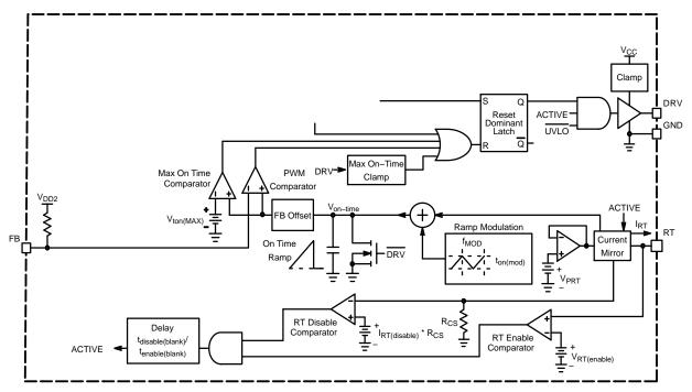
Figure 4. On-Time Control Architecture
