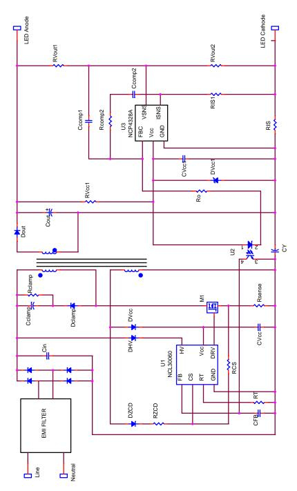
Figure 1. NCL30060 Typical Application Diagram
