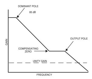
Figure 1. ILC7083/ILC7084 RF LDO Frequency Response
