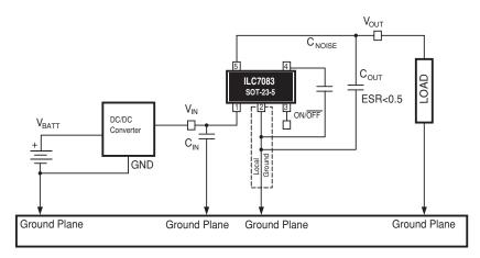
Figure 8. Recommended Application Circuit Schematic
