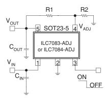
Figure 3. Application Circuit for Adjustable Output Voltage
