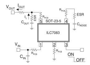
Figure 6. Inherent PCB resistance
