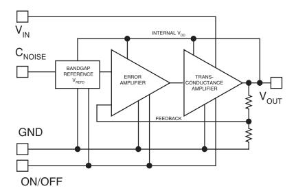
Figure 2. ILC7083 RF LDO Regulator Block Diagram
