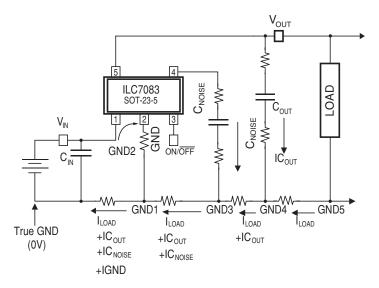
Figure 7. Effects of Poor Circuit Layout
