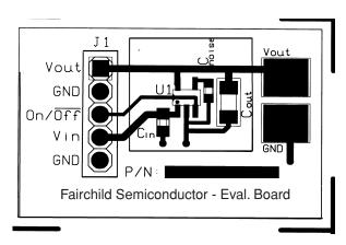
Figure 9. Recommended Application Circuit Layout (not drawn to scale)
