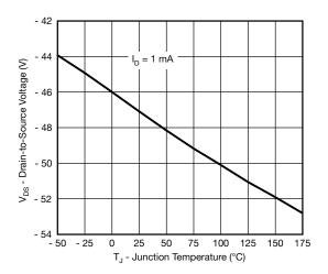
**Drain Source Breakdown vs. Junction Temperature**
