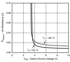
On-Resistance vs. Gate-to-Source Voltage
