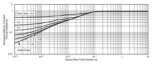
Normalized Thermal Transient Impedance, Junction-to-Case
