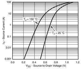
**Source Drain Diode Forward Voltage**
