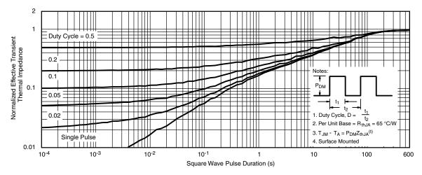
Normalized Thermal Transient Impedance, Junction-to-Ambient
