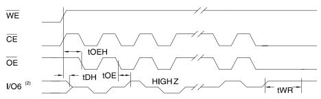
Notes: 1. Toggling either  $\overline{OE}$  or  $\overline{CE}$  or both  $\overline{OE}$  and  $\overline{CE}$  will operate toggle bit.
